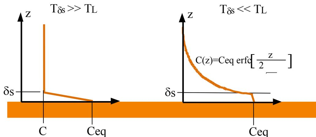
**Figure 4.** Distribution of concentration near a dissolving boundary for conditions with slow transport across the laminar sub-layer ( $T_{\delta_s} \gg T_L$ ) and conditions with rapid transport across the laminar sub-layer ( $T_{\delta_s} \ll T_L$ ).
