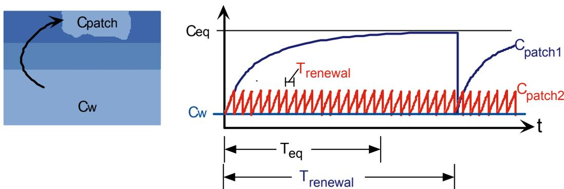
**Figure 7.** For case 1 (blue curve) the renewal time scale is longer than the equilibrium time-scale. For case 2 (orange curve) the renewal time scale is much shorter than the equilibrium time-scale. Greater flux is achieved in case 2, because the average concentration gradient across the interface ( $C_{\text{patch}} - C_{\text{eq}}$ ) is larger.
