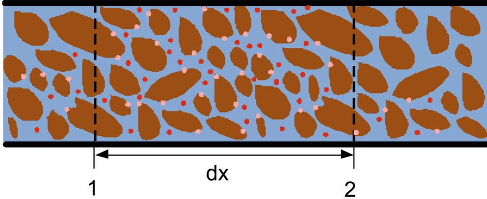
**Figure 9.** Boundaries at 1 and 2 define a one-dimensional, sub-surface control volume with cross-sectional area  $A$ . The soil matrix is shown in brown and the groundwater in blue. The chemical mass is partitioned between the water phase (red dots) and the solid phase (pink dots). At equilibrium the ratio of concentrations in the solid phase ( $C_s$ ) and water phase ( $C_w$ ) is given by the partition coefficient,  $K_d = C_s/C_w$ .
