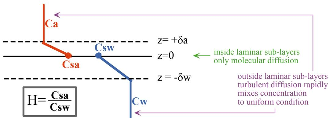
**Figure 5.** The Thin-Film Model describes the exchange of volatile species across the air-water interface under conditions for which transport is limited by diffusion across the laminar sub-layers. At the surface ( $z = 0$ ) the aqueous phase ( $C_{sw}$ ) is in equilibrium with the concentration in air ( $C_{sa}$ ), such that  $C_{sw} = C_{sa}/H$ , where  $H$  is the Henry's Law constant.
