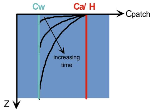
**Figure 8.** Diffusion of mass into a new patch brought to the surface at  $t = 0$ . Before patch arrives at surface ( $t < 0$ ),  $C = C_w$  throughout the patch. For  $t \geq 0$  the concentration at the patch-air interface ( $z = 0$ ) is at equilibrium with the air,  $C_a/H$ .
