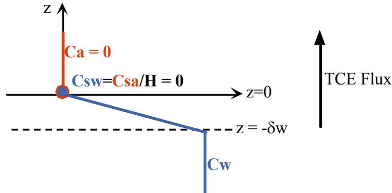
**Figure 6.** The flux of TCE from lake to atmosphere is controlled by the water-side laminar sub-layer. The air-side laminar sub-layer is negligible so that  $C_{sa} = C_a$ . Furthermore, since  $C_{sw} = C_{sa}/H$ ,  $C_{sw} = 0$  as well.
