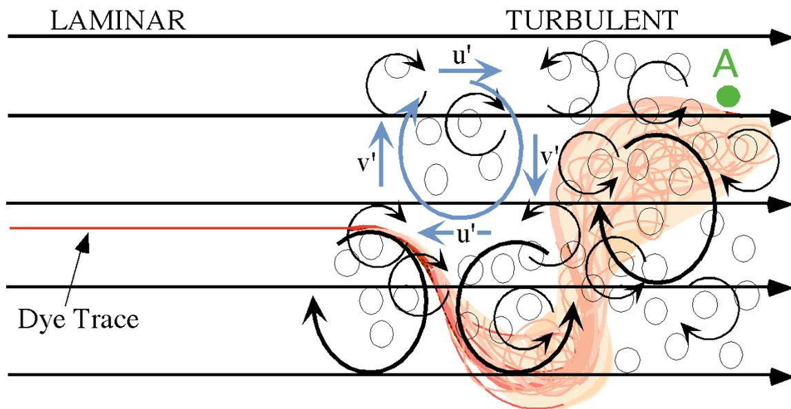
**Figure 1.** Tracer transport in laminar and turbulent flow. The straight, parallel black lines are streamlines, which are everywhere parallel to the mean flow. In laminar flow the fluid particles follow the streamlines exactly, as shown by the linear dye trace in the laminar region. In
