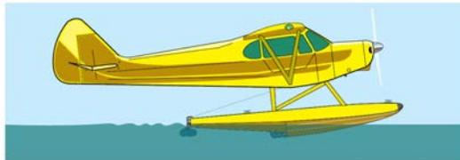
Figure 4-6. Plowing position.
