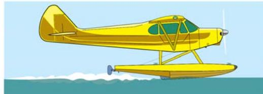
Figure 4-7. On the step. The altitude is nearly level, and the weight of the seaplane is supported mostly by hydrodynamic lift. Behind the step, the floats are essentially clear of the water.
