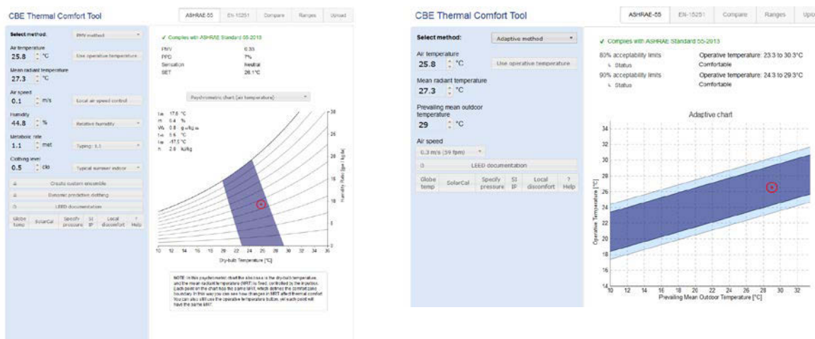
Figure: Thermal comfort conditions according to PMV (top) and Adaptive Comfort theory (bottom)
