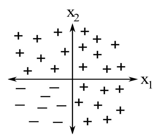
The neural net is supposed to output a positive value for the data points marked +, and a negative value for the data points marked -. Lyla finds that no matter what initial weights she uses, and how and how much she trains the neural net, its error rate on the training data never goes below about 1/8. Why?
