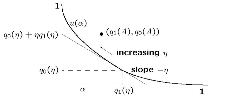
If the vertical axis of the error curve is inverted, it is called a receiver operating curve (ROC) which is a staple of radar system design.
