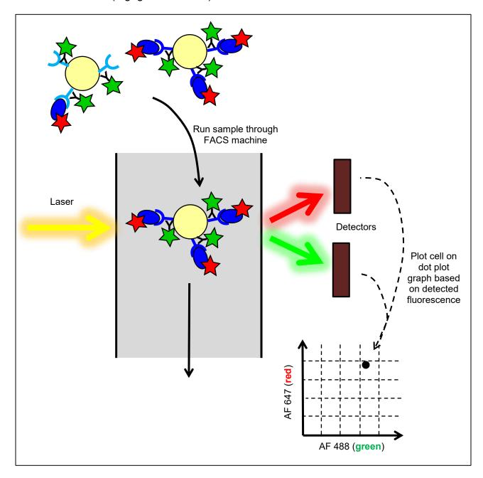
**Step 4a:** Sort the cells as they pass through the FACS machine based on the level of fluorescence per cell for each of the measured color channels. You can arbitrarily set a pre-defined range or "gate," where all cells that have fluorescence levels that fall within that gate are sorted and saved into a tube.
