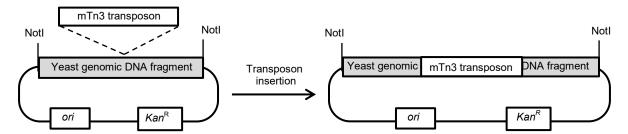
**Figure 1.** Yeast transposon library plasmid containing a fragment of yeast genomic DNA in which a mTn3 transposon has been randomly inserted. The plasmid backbone (the Notl-to-Notl portion containing the *ori* and *Kan*<sup>R</sup> sequences) is 2.1 kb in length.
