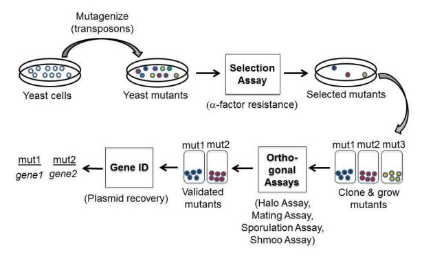
**Figure 1.** Overview of a forward genetics screen. (Figure adapted from Omer Yilmaz 7.02 Spring 2019 lecture slides.)
