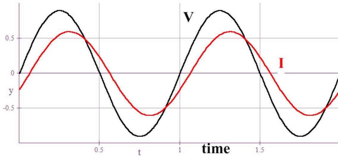
The plot shows the driving voltage  $V$  (black curve) and the current  $I$  (red curve) in a driven RLC circuit. In this circuit,
