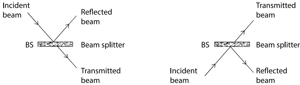
Figure 3: An incident beam hitting a beam-splitter results in a reflected beam and a transmitted beam. Left: incident beam coming from the top. Right: incident beam coming from the bottom.
